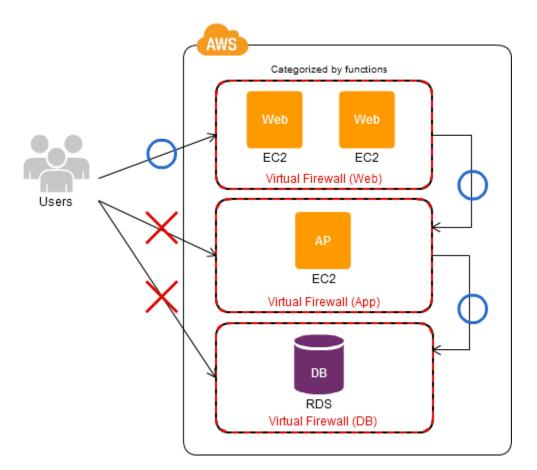
Multi-tier access control improves security. The EC2 virtual servers are grouped by individual functions, eliminating the need to change the virtual firewall settings even when using the scale-out pattern.
