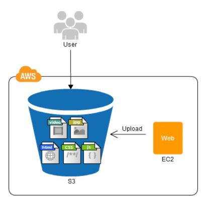
• Access to the static content is left to S3, enabling you to increase the the availability and durability of the web system with ease.
