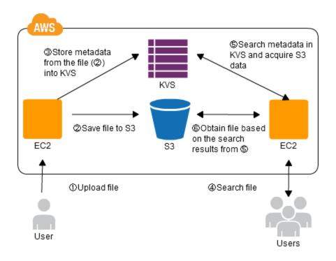
• This enables you to use robust high-capacity storage functions along with high-performance searching.
