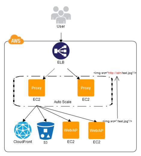
• Overwriting the access destinations using a proxy server makes it possible to distribute the load of static content without modifying the existing system.
